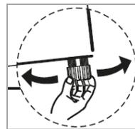
Check with a spirit level whether the appliance is leveled horizontally. If the unit is not in balance, the feet must be adjusted.
